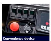
A lamp switch and an emergency switch, installed at the right side of the dashboard, cut power in emergencies and enhance operability. A USB port is also added to enable users to recharge their portable appliances.
