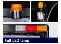
The long-lasting, high-illumination full LED working lamp (front & rear) and combination lamp enhance safety and working efficiency when operating at night or in darkness. Also, the standard warning light provides workplace safety.
