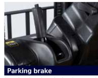
New hand parking brake device with release button greatly reduces fatigue in operation.
