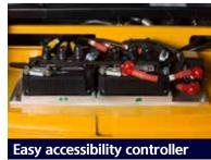
The traction and pump controllers can be accessed by removing the top cover of the counterweight. The controller is installed horizontally to ensure easy repair, and the top cover blocks dust and moisture.
