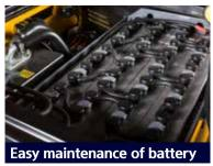
The battery cover opens fully with the assistance of a gas strut that locks when fully opened to give easy access to battery and prevent the hood from dropping. An automatic electrolyte liquid filling machine is offered as an option for hassle-free battery maintenance.
