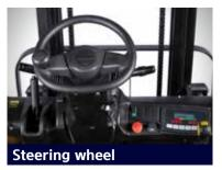
The angle of the steering column can easily be adjusted to improve operator
