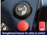
The emergency switches enable the operator to respond quickly in an emergency. Also multifunctional graphic display indicates the vehicle's status.
