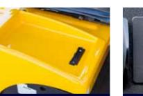
Urethane bolt minimizes battery movement and fastens battery cover on the right side of the frame for safer operation.
