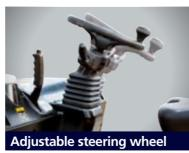
The steering handle can be adjusted forward/ backward using the lever on the bottom of the column.
