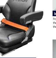
• ELR (Energy Locking Retractor) type seat belt • Heater and Backrest extension (OPT)
